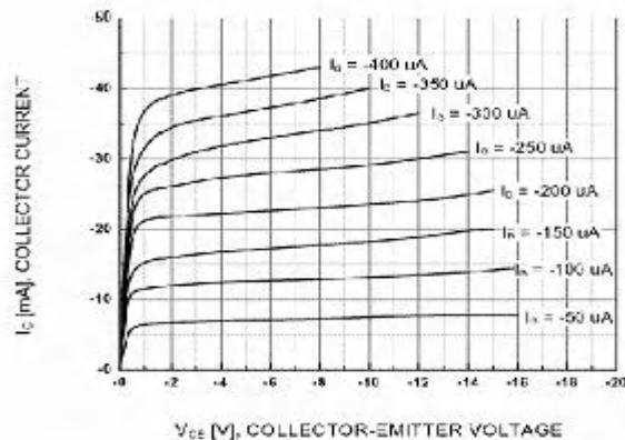
Figure 1. Static Characteristic
